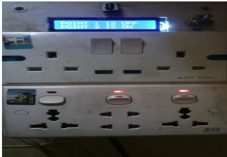
Figure 6: Point 1 OFF and Point 2 ON
