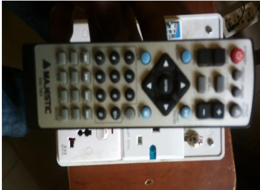
Figure 3: Remote Control (IR transmitter) and the constructed circuit
